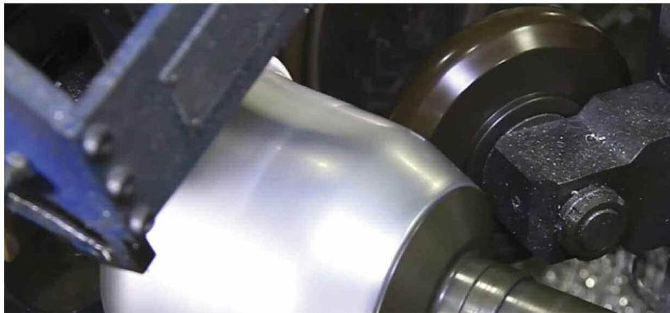
*Compared to metal spinning wheels, the polymer wheels run on Reflek’s spinning machines boast better hardness and wear characteristics, and better maintain their machined shape to promote long production runs and minimal downtime.*
