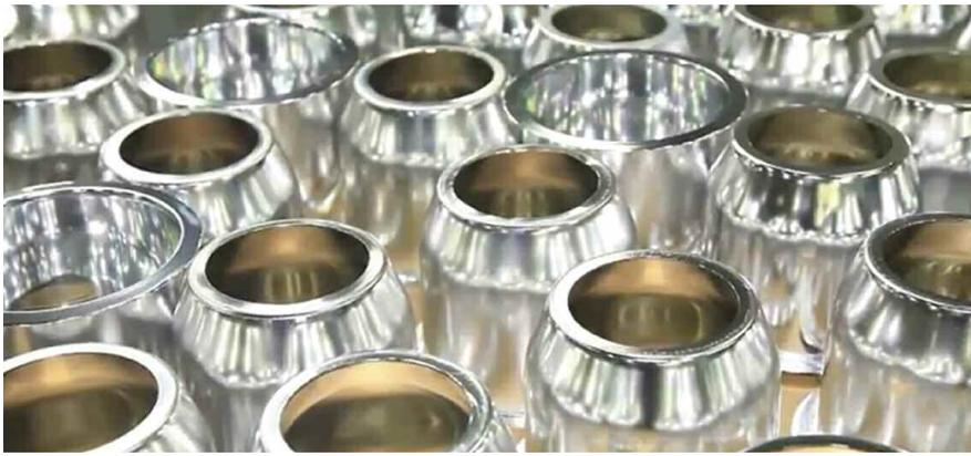
Due to the trend toward LED lighting in commercial and residential applications, aluminum reflectors (shown here) tend to be circular. That makes metal spinning the manufacturing process of choice at Reflek Manufacturing, where “the combination of our high-quality spinning machines and the Boedeker polymer wheels are the only way we can achieve the consistency of surface finish we and our customers desire,” says Reflek’s Alan Dorsky.
